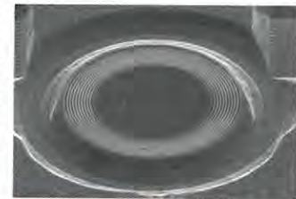
SUNNY SIDE UP Concentric ridges make light waves in this light-emitting diode (raised central plateau) bend upward, boosting the diode's brightness.
