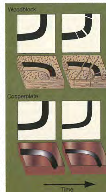
TIME'S IMPRINT — A carved woodblock (top) dries out and cracks between print runs, resulting in broken lines in subsequent prints. Scouring away corrosion on a copper plate (bottom) wears down the metal and may narrow engraved grooves, causing thinner lines in later prints.
