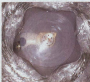
CURRENT EVENT A whirlpool, viewed from above, takes a pentagonal shape just above the spinning platter that's causing the water to swirl.
