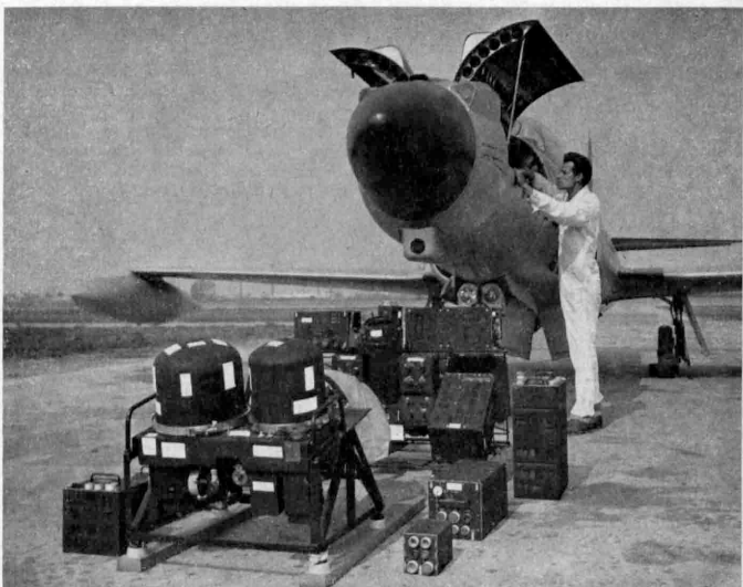
DISSECTED "BRAIN" — Electronic "seek-and-kill" equipment, like that now installed in all U. S. and Canadian interceptor planes defending the continent against air attack, is displayed. The gear takes over control of the craft 15 miles from target and fires rockets automatically. The display includes as many parts as 200 television sets.
