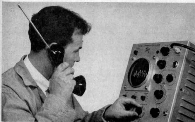
NO BATTERIES —Experimental model of a voice-powered radio transmitter is tested by its developer, George Bryan, of the Signal Corps Engineering Laboratories. Notice no wires dangle from the telephone receiver in which the device is installed.
