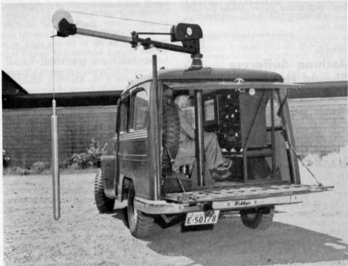
GAMMA RAY LOGGING UNIT —To aid in prospecting for radioactive minerals, including uranium, this jeep-mounted unit is equipped with a scintillation counting probe, more sensitive than a Geiger counter.
