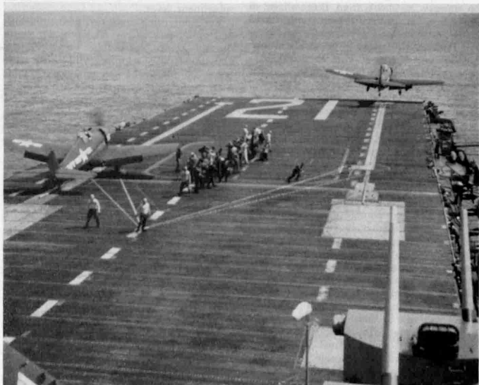
LAUNCHING ROBOT PLANE—An AD-2 guide plane at the right of the photo is taking off from the deck of the USS Boxer. At a designated spot it will take control of the robot plane, the F-6-F shown on the left receiving a final instrument check. Equipped with special electronic gear and armed with a powerful warhead, the drone plane can be directed to its objective by the control plane which remains many miles away and high above the flock.
