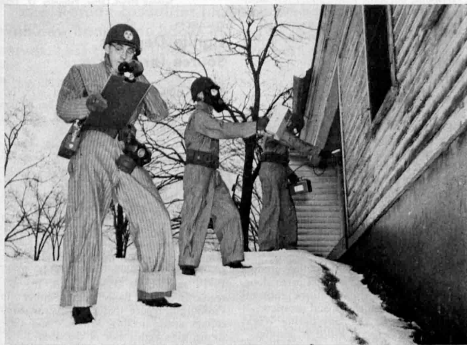
RADIATION DETECTION —This "emergency team" is demonstrating how radioactivity could be measured in case of an atomic blast. The team is from the Knolls Atomic Power Laboratory of General Electric. The man in the foreground records readings reported by the other two and radio-telephones the information to a central plotting point.
