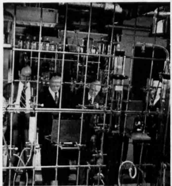
INSIDE THE MILK INDUSTRY— Ion exchange columns in the chemical laboratory of the new National Dairy Research Laboratories are the apparatus used to remove mineral salts and acids from whey. These laboratories are at Oakdale, Long Island.
