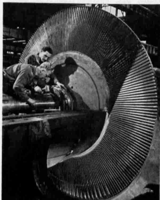
ELECTRICITY FOR 300,000—A modern General Electric turbine, 12 times more powerful than the first of the "big" turbines, is shown under construction in Schenectady. With improved design and increased size, a single modern turbine may provide enough electricity to supply the normal electrical requirements of a city of 300,000 people.
