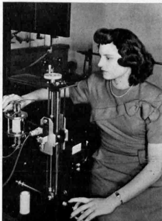
X-RAYING OIL FIELD —A sample of field rock is mounted in the apparatus where it is injected with oil, gas and water and then X-rayed. This reveals the behavior of fluids in the rock formation. The process is expected to net a greater percentage of oil.
