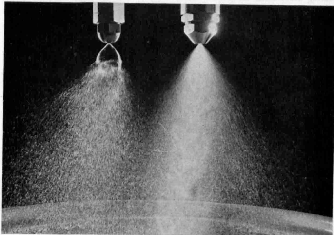
FUEL ATOMIZER —The new type nozzle, right, sprays oil in a miniature cyclone of vapor particles. It is compared to the conventional nozzle on the left.
