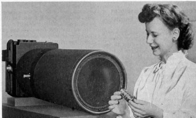
TELEPHOTO LENS —With this 125-pound lens, the Army Air Forces will be able to snap large, sharp pictures from altitudes as high as 10 miles. The lens, compared in the picture to a lens like in a 16-mm. movie camera, is a foot in diameter and four feet long.
