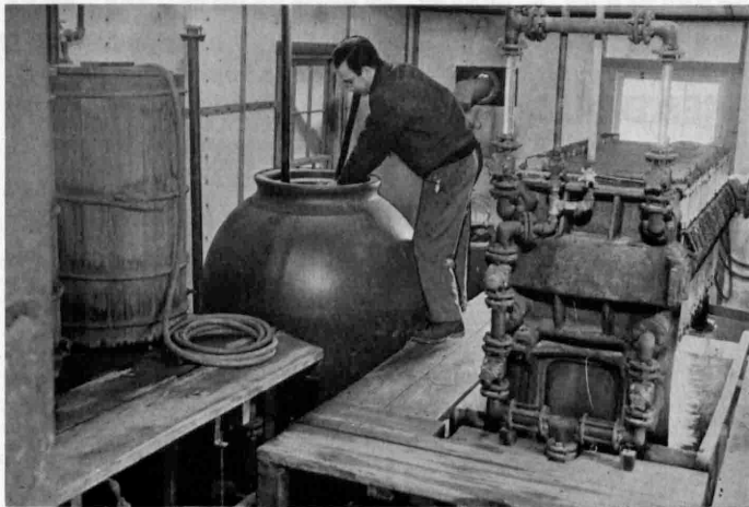
IN SOLUTION—Silica and other insoluble matter are removed from the aluminum by a filter press.
