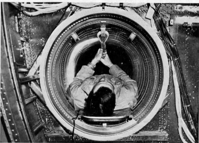
BOMBER SUBWAY —To get from one compartment to another in flight on the mammoth XB-36, crew members must ride a miniature subway. The tunnel is two feet in diameter and 85 feet long. A scooter, propelled by an overhead cable, is the subway "car".
