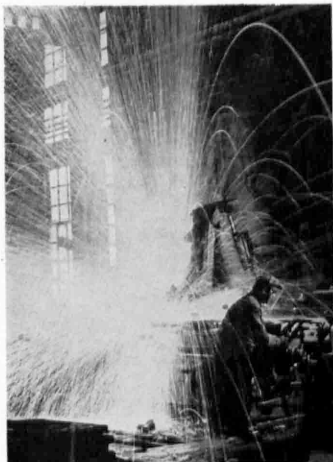
SPARK SHOWER —Two ends of a rotor ring for a huge generator are being melted in a General Electric laboratory for welding together at temperatures approaching 3,000 degrees Fahrenheit. The apparent shower is caused by the fact that sparks and molten steel particles move too fast for the camera.
