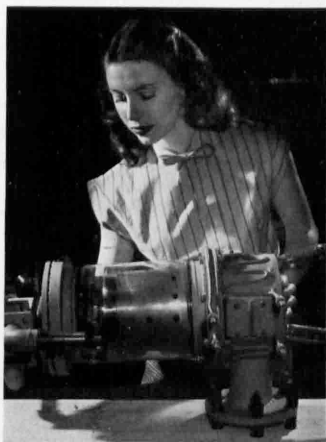
RADAR JAMMER —The world's heaviest and most powerful micro-wave tube, the resnatron, is being modified at Westinghouse Laboratories to improve television and ultra-high frequency transmission.
