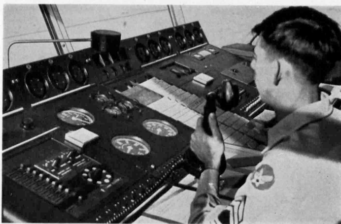
CONTROL TOWER CONSOLE —This unit, developed by the Army Air Forces for air safety, incorporates all the utilities necessary to control air traffic that have been scattered throughout the tower.
