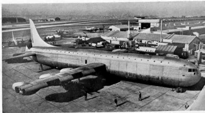
XC-99—World's largest land-based aircraft, the Army Air Forces' XC-99 cargo and troop transport is nearing completion at Consolidated Vultee's plant in San Diego, Calif.
