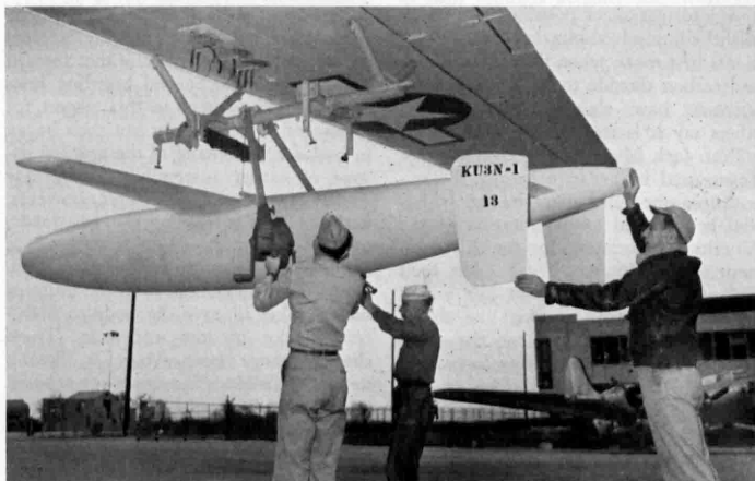
REMOTE CONTROLLED —KU3N-1 is an air-to-ground missile, launched from under the wing of its parent airplane and flown by remote control from another plane. This missile can reach its target at speeds greater than 500 miles per hour. Official U. S. Navy Photograph.
