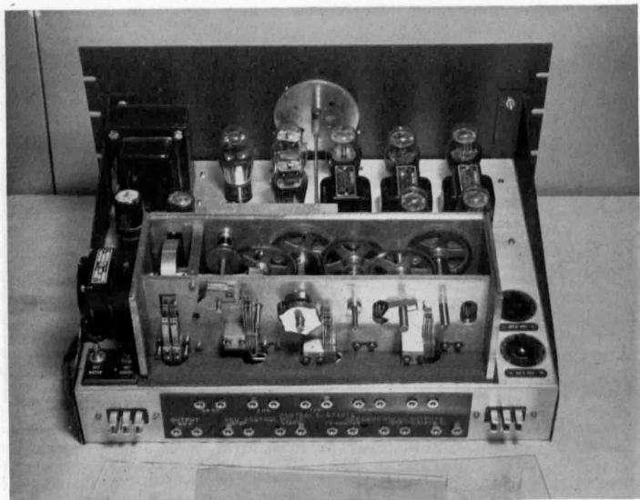
HELPING IT TICK —Rear view of the National Bureau of Standards seconds pulse generator and time interval selector used in the time control equipment of the Bureau's radio station WWV.
