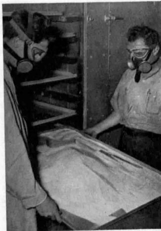
**JUST PILLS**—Workers making the new antimalarial take dried Aralen crystals from oven for transfer to tablet-making machine in the Winthrop Chemical Co. laboratory.
