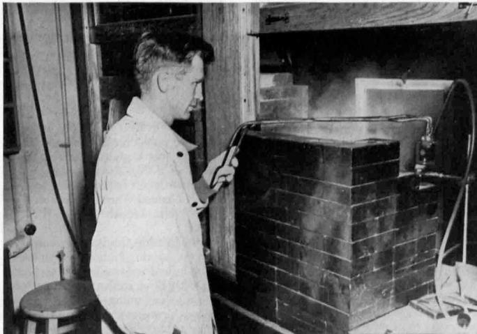
**OAK RIDGE**—Lead bricks absorb radiations from the material in the beaker, in this laboratory at Oak Ridge, Tenn. The chemist watches his work in the mirror and handles the apparatus with a relatively short pair of tongs. Equipment of this type is used in the production of radioactive materials.
