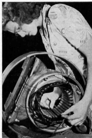
ELECTRIC MOTOR —Wire coils are being installed in the stationary part of one of the new all-steel-encased motors under construction in the Buffalo plant of the Westinghouse Electric Corporation.
