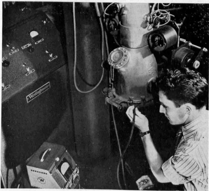
LEAK DETECTOR —Tiny leaks in the vacuum systems used in atomic research and other electronic and chemical processes can be detected by this device, developed by Westinghouse. If there is a leak, helium gas will enter the system and be detected by a sensitive electronic tube in the large black unit at the left. The amount of helium entering the vacuum system will be recorded on the meter dials, indicating the size of the leak.
