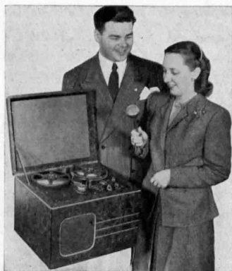
HOME RECORDER —Radio programs, speeches and greetings to friends may be recorded on paper tape in this set designed for home use.
