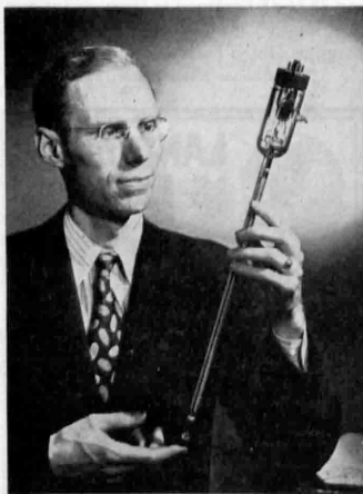
100,000,000 WORDS A MINUTE— This new and simple vacuum tube amplifier developed by Dr. John R. Pierce of Bell Telephone Laboratories (holding the tube) may have far-reaching significance in long-distance telephone and telegraph transmission.
