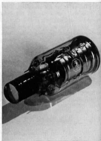
NIGHT EYES —This RCA Type 1P25 infra-red light tube was the eye of the electron telescope used by the Navy to conduct landing, reconnaissance and offensive operations as well as code communication by blinker lights under cover of absolute visual darkness.
