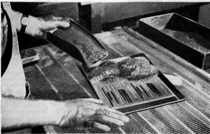
PLASTIC GRANULES —These are spread on the matrix before it is inserted into the press, where it is heated and squeezed to take the form of the original printing plate.
