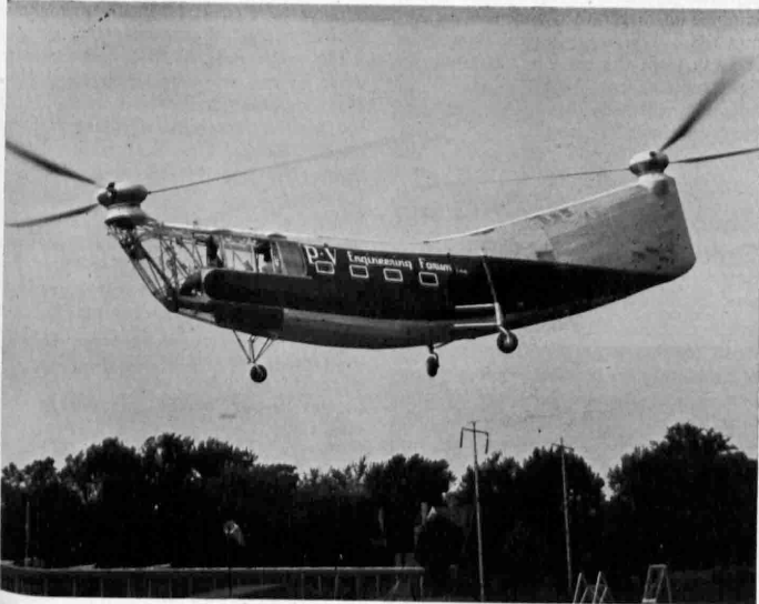
LARGEST HELICOPTER —The PV-3, manufactured by the P-V Engineering Forum, Inc., is shown in flight over the company's Sharon Hill, Pa., plant. The machine is being readied for production as the latest Navy-Coast Guard air-sea rescue and special transport vehicle. It is the first transport type helicopter.
