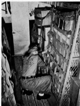
ZIPPED IN —This shows how the cargo is held in place in the Airfreighter. The packages are zipped, buckled or strapped into the separate bins to keep them from shaking while in the air
