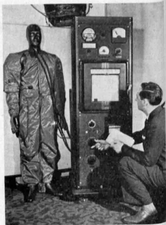
COPPER MAN —He will save human volunteers from the suffering of low temperature tests of electrically warmed clothing for the armed forces. Robert Sambleton, General Electric engineer, makes notes as the copper robot reproduces the human temperature system.
