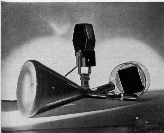
CARRY SOUND AND LIGHT —Modern devices enable electrons to carry sound and light to distant places. The funnel-shaped tube is a cathode-ray tube on which pictures in your television receiver will appear. The microphone picks up words and music. The tube at right is the electronic kinescope which picks up pictures in the television camera for transmission to your home.
