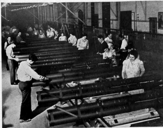
**FLYING BAZOOKAS**—The air-minded cousin of the famous infantry gun is made on a mass-production basis at the plant of the General Electric Company. The rocket tubes are mounted in groups of four under the wings. See *SNL*, July 15, for a photograph of the rockets in flight.
