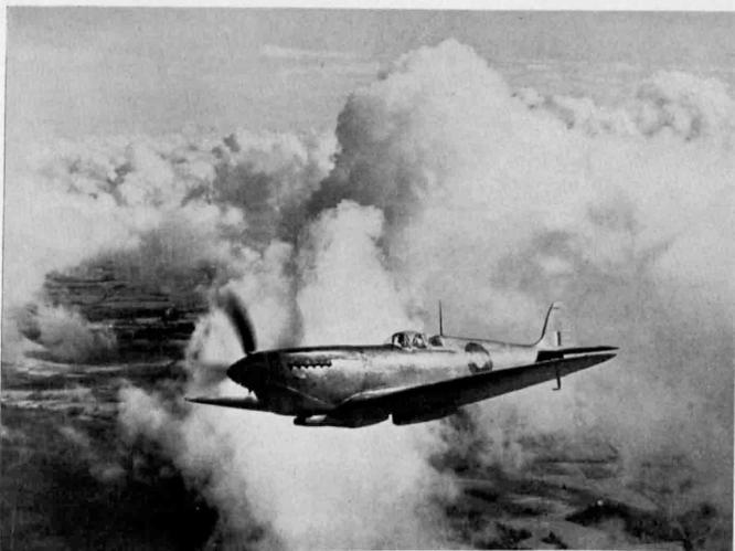
ARMY "EYES"—The Spitfire, shown in this official British photograph, is an all-metal single seat, low wing monoplane, specially designed for photo-graph reconnaissance duties. The cameras are fitted in the fuselage.
