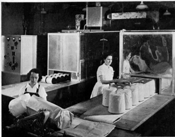
PERMANENT SET —With this electronic heating equipment, 18-pound cones of rayon tire cord are treated in a high frequency electrical field to make its twist lasting.
