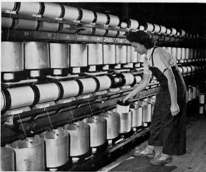
TWISTING —Production of tire cord requires two twisting operations. This is the second step, in which twisted threads from two bobbins are cable twisted into finished cord. This photograph was made at the plant of the Industrial Rayon Corporation.
