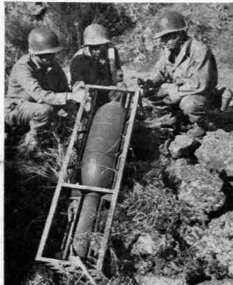
FIERY MISSILE —With Nazi propagandists busily spreading dark hints about "secret" super-rockets intended to soar across the Channel and blast Britain, unusual interest attaches to this picture taken in Sicily by the U. S. Army Signal Corps. It is of a captured German incendiary rocket of 32 centimeter (12.6 inch) caliber. The framework in which it rests serves both as shipping crate and launching cradle. It is shown here in firing position.
