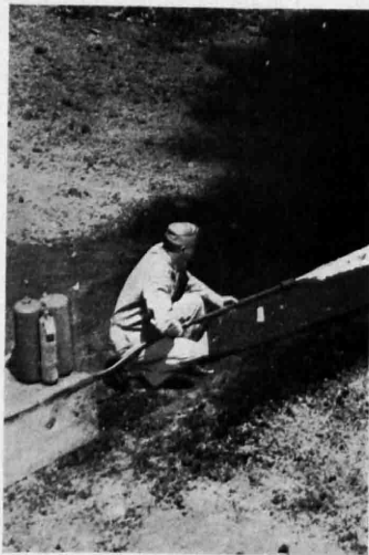
FLAME THROWER —The two large tanks of the apparatus contain enough fuel for several shots of flame. Two are used instead of a single large tank to reduce the soldier's silhouette, making him a smaller target. The third tank contains inert gas to provide pressure. Rubber hose connects the tanks to the "gun," a metal tube about four feet long with a nozzle inside near the front end.
