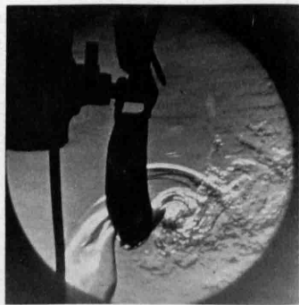
HOT AIR —This is what happens when a stream of hot air hits an electric fan revolving at 1800 r.p.m. It was pictured at the general engineering laboratory of the General Electric Company with a high speed camera, using an exposure of about 1/2,000,000 second
