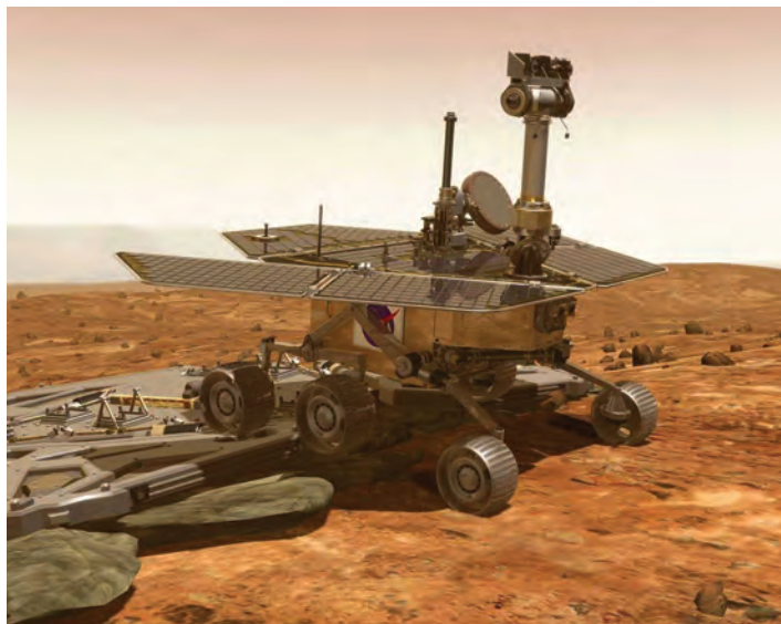
RED ROVING — After bouncing to a stop, the lander's petals will unfold and the Mars Exploration Rover will drive onto the surface.
