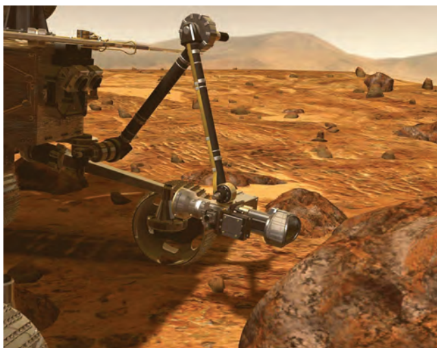
ROCK SCRAPER — The abrasion tool, located on the arm of each of NASA’s twin robotic landers, can remove a nickel’s thickness of material from a rock so that spectrometers and other instruments can explore the sample’s interior.
