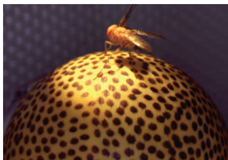
FLY BALL — A Ping-Pong ball painted with dots provides a monitor of how a tethered Ormia fly tracks sounds. Optical sensors picked up the shifting of the dots and sent the information to a computer.
