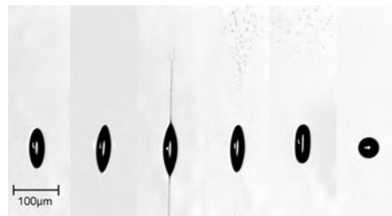
FREEZE FRAME Six droplets, photographed at increasing time intervals after instability, show the development of Rayleigh jets (third image) and their disappearance.
