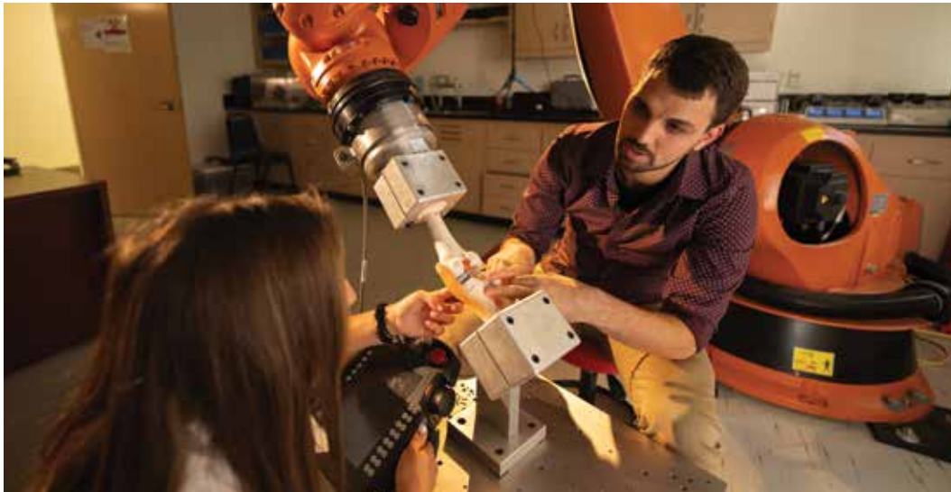
In their lab at UCLA, bioengineer Tyler Clites and Ph.D. candidate Ophelie Herve use a robot arm to manipulate a model knee in a simulation of an experiment to be conducted on cadavers.
