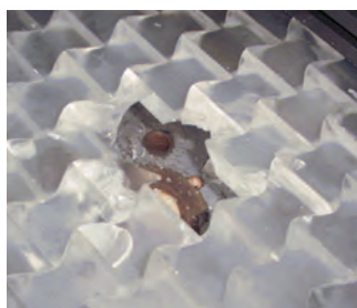
HARD HIT Missing blocks show where a steel shaft struck a test panel of interlocking but unglued epoxy-resin blocks. Outside the impact zone, the panel remained intact because cracks couldn't spread from block to block.
