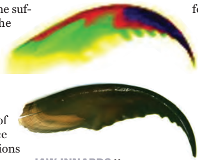
JAW INNARDS X-ray absorption (top) shows the highest concentration of zinc (dark area) near the tip of a clam-worm jaw. A light-microscope image of the jaw, about 3 millimeters long, appears at bottom.
