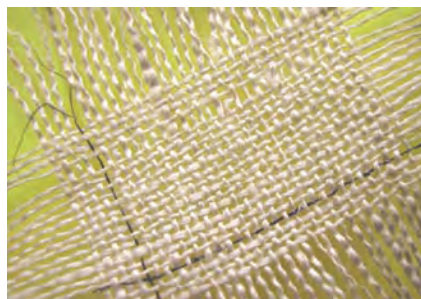
FUTURISTIC FIBERS Materials scientists used carbon nanotubes to make two electricity-storing supercapacitors (black threads) that they inserted into cloth. The woven area is a little more than 2 centimeters long.
