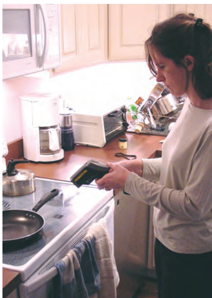
HOT STUFF A researcher uses a gun-style, noncontact thermometer to take the temperature of a PTFE-coated pan.
