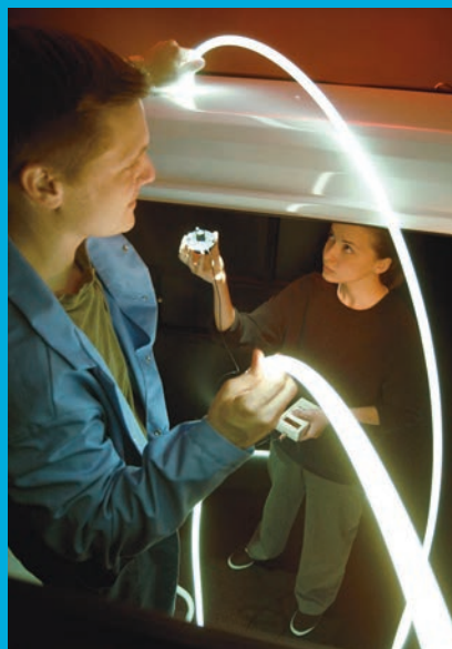
HYBRIDIZED — Sunlight collected by the large mirror (top) is focused into a smaller one above it and then reflected down through a rooftop opening into a bundle of optical fibers. Routed to ceiling fixtures (bottom), the fibers light up an acrylic rod that's placed between fluorescent tubes. When the sunlight and fibers are bright, the fluorescent lights cut their output.
