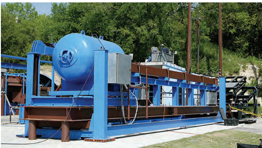
BIG GUN Compressed-gas gun at Southwest Research Institute in San Antonio that's used to shoot chunks of shuttle foam at targets resembling shuttle coating.
