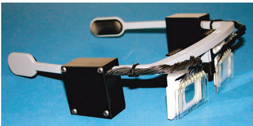
LOOK OUT Electric signals from microchips in the black boxes attached to these prototype eyeglasses change focus settings to improve near vision.
