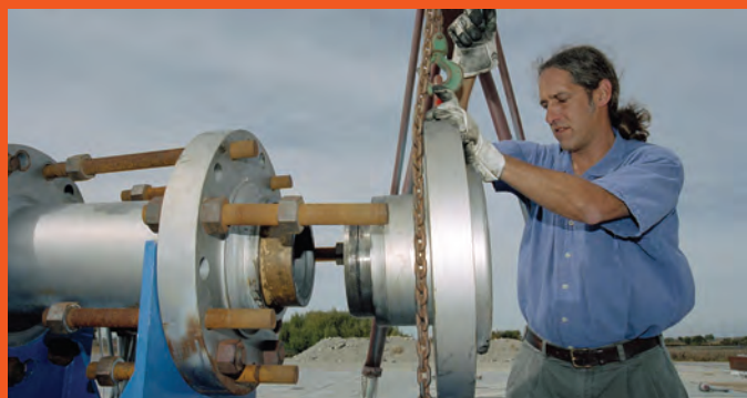
WAX WORKS — Stanford researcher Arif Karabeyoglu installs a cardboard tube of paraffin-based fuel into the combustion chamber in NASA Ames' Hybrid Rocket Test Facility (top). Ames engineer Greg Zilliac seals the test chamber.
