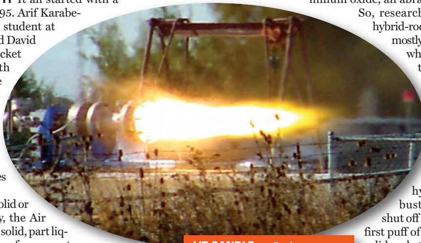
LIT CANDLE — Engineers test-fire a rocket containing a paraffin-based hybrid-rocket fuel.
