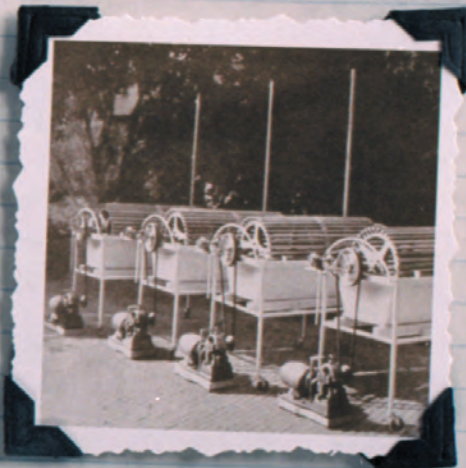
Artificial kidney, 1947. Dr. Willem Kolff's first kidney dialysis machine, invented in the early 1940s, used cellophane tubing made for sausage casings.
