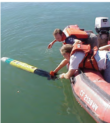
CIRCUITS OVERBOARD — Battery-powered torpedoes such as this REMUS can map the ocean floor, measure the salinity or speed of ocean currents, or sniff the water for particular chemicals.
