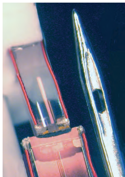
CHEAP FIX Smaller than a needle (right), a liquid-crystal and gold device tucked between these glass blocks tunes up signals passing through the optical fibers encased in the blocks.
