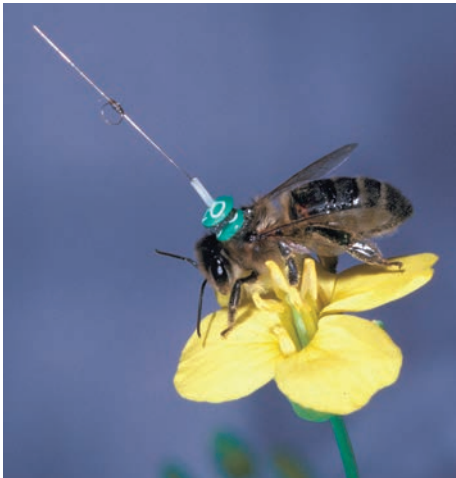
BEE WHERE — The device fastened to the back of this insect changes an incoming radar frequency in a predictable way and reflects it. Trackers at ground level listen for the predicted frequency and ignore the chaos of other reflected signals.
