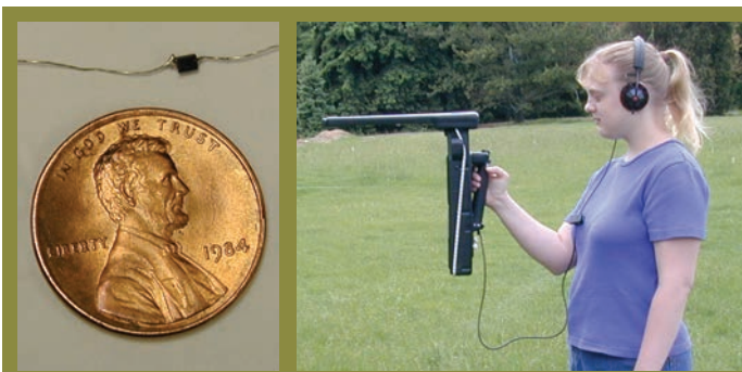
START SMALL — A diode (the rectangle above the penny in the image on the left) responds to harmonic radar but is small enough for an insect to wear. Wires attached to the diode serve as an antenna. No batteries required. A woman (right) holds a commercial direction-finding device that sends out a signal and listens for a particular multiple of that signal bouncing back. Designed for rescue work, the device has been modified to look for insects.
