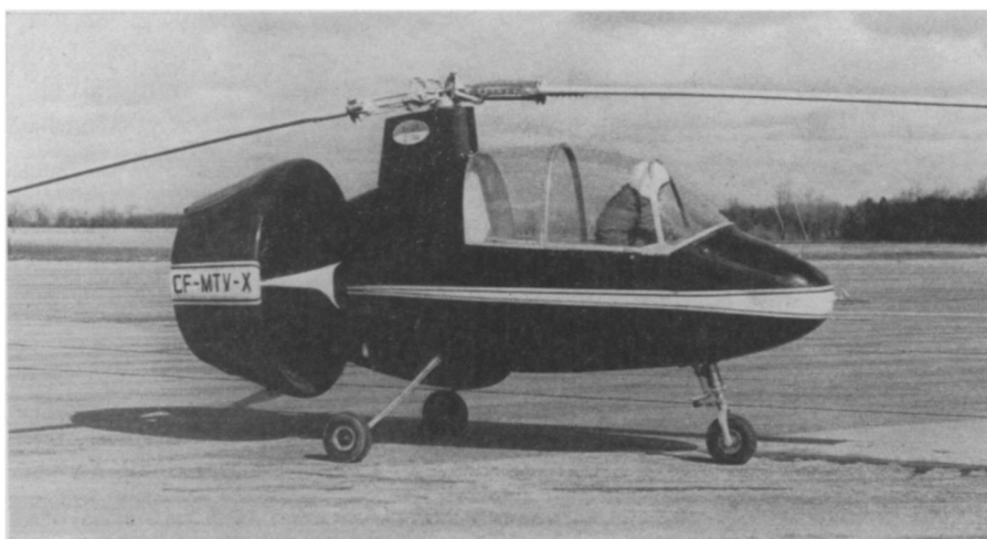
LIGHTWEIGHT PLANE —A thin skin of polyester resin and fiberglass covers the Avian 2/180 gyroplane. The covering, having unusual strength and light weight, was made by the Hooker Chemical Corporation, Niagara Falls, N. Y.
