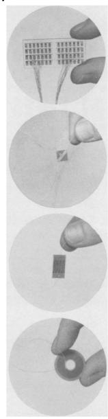
We make Kodak Ektron Detectors like these for transducing a visible or infrared pattern into electrical terms. The darker material is photoconductive lead sulfide or lead selenide; the electrodes (actually evaporated gold) appear grey here. Since we can lay down the photosensitive material in any configuration, enormous potentialities for inventiveness present themselves. Whether you seize them is entirely up to you. We offer a pamphlet,
