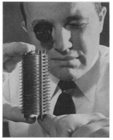
ROBOT READER—This laminated iron and copper unit is the "eye" and "hand" of a new data-processing system designed by Datamatic Corp., Newton Highlands, Mass. Magnetic tape storing the information passes over the device shown here, at a rate of 100 inches per second.
