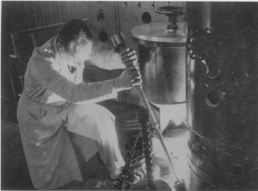
METAL PURIFIER —An operator checks the temperature of a molten alloy in the new, 1,000-pound vacuum melting furnace now in operation at the Carboly Department of General Electric Company in Detroit. The furnace is used to make the purest possible metals and alloys for use in such devices as gas turbine autos, now bottlenecked because of costly materials.
